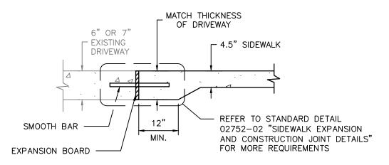
DETAIL D4 DRIVEWAY/SIDEWALK HEADER
