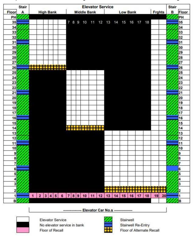
Example No. 2 – Elevator Riser Diagram: Elevator and Stairwell Diagram
