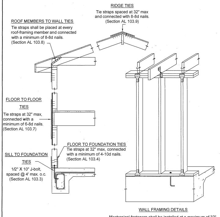
Mechanical fasteners shall be installed at a maximum of 32" o.c. to connect studs to top plates, sole plates and sill plates Fasteners shall be nailed with a minimum of 8-8d nails. (Section AL 103.5)
