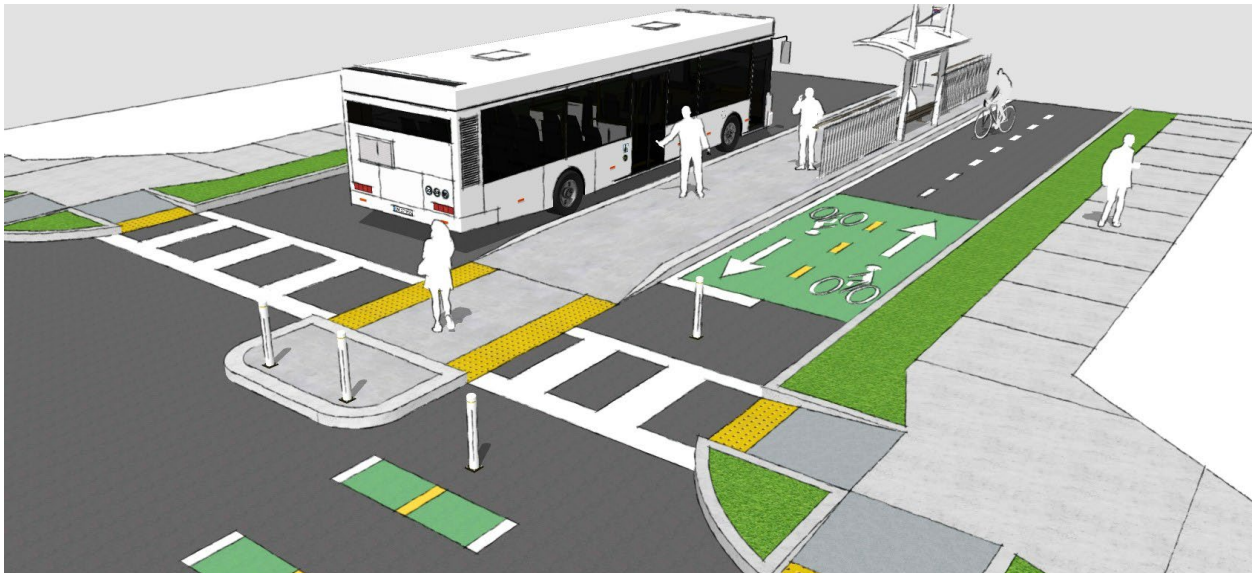
Figure 17.29 – FLOATING BUS STOP B
