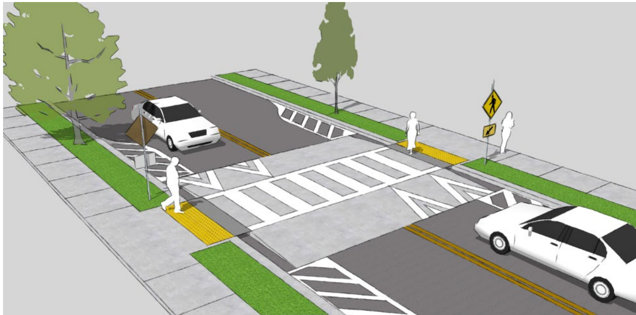
Figure 17.12 - RAISED CROSSWALK ON A TWO-WAY, UNDIVIDED ROADWAY
