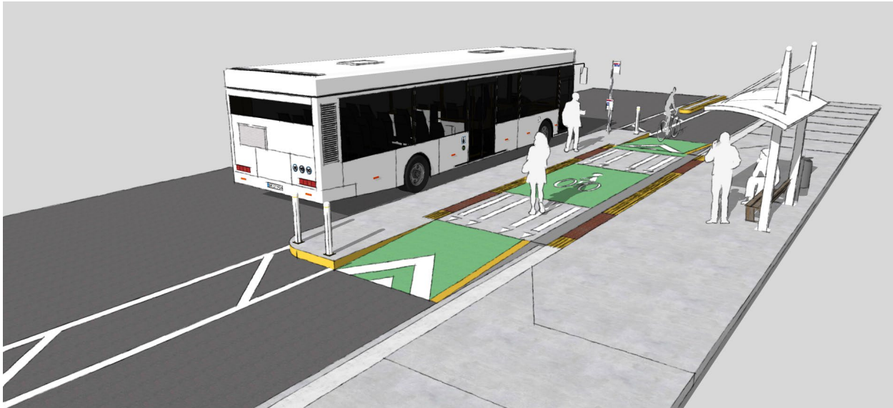
Figure 17.30 - SHARED RAISED BUS STOP
