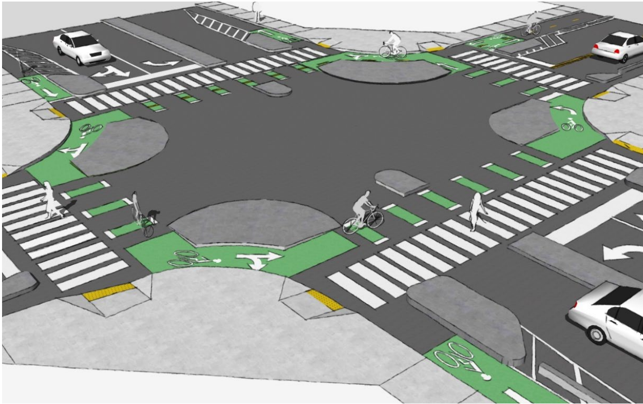
Figure 17.26 - PROTECTED INTERSECTION (RETROFIT)
